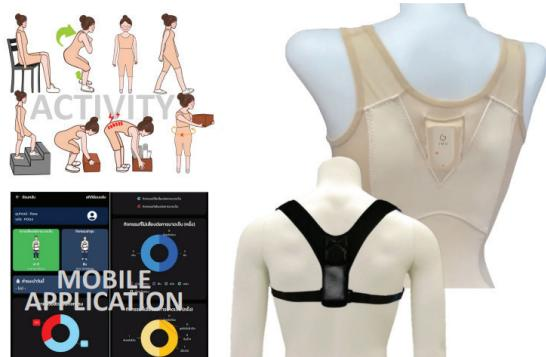
This is a wearable device using artificial intelligence (AI) technology to monitor, predict, and alert risks from improper movements and falls. The system sends alerts to caregivers. It is lightweight, easy to use, can be worn all day, and is designed to fit the Thai body structure.
