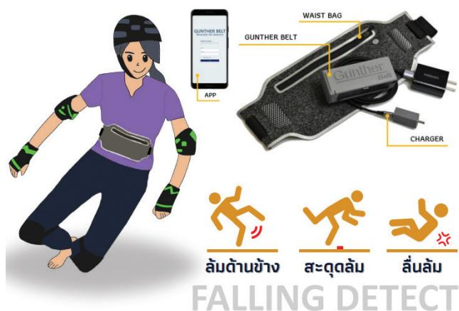
This innovation can detect falls immediately and transmit signals via NB-IoT (Narrow Band Internet of Things) directly to a server without requiring a gateway device. It has a battery that lasts at least 3 hours and features a display screen for caregivers to monitor user falls.
