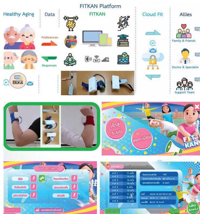
This innovation is a wearable exercise measurement device that uses sensors and wireless processing, incorporating AI to record and provide a preliminary evaluation of an older person's physical activity. It delivers appropriate and diverse information, tracks progress over time, and allows effective use of data for health management. The system includes role-based access control for administrators, staff, health managers, nurses, and the older persons themselves.
